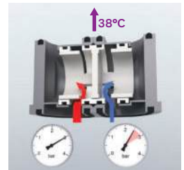
At 38°C: HW 3 bar/CW 2.5 bar
