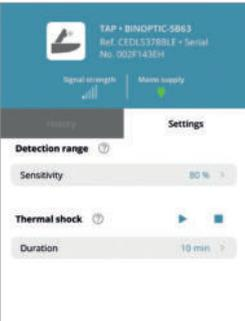
The **detection distance** can be set by adjusting the sensitivity of the sensor to the washroom surroundings (position, washbasin height, etc.).
